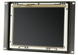
KE097 is a cost-effective, high-quality open frame LCD monitor suitable for integration with any industrial or commercial application. KE097 features 1024x768 with wide view angle of 170(V)/170(H) degree and LED backlight IPS LCD panel, which saves more energy and lasts significantly longer than conventional CCFL backlights.
