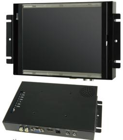
KE082 is a cost-effective, high-quality open frame LCD monitor suitable for integration with any industrial or commercial application. KE082 features 800x600 resolution with wide view angles of 120(V)/140(H) degree and LED backlight TFT LCD panel, which saves more energy and lasts significantly longer than conventional CCFL backlights.
